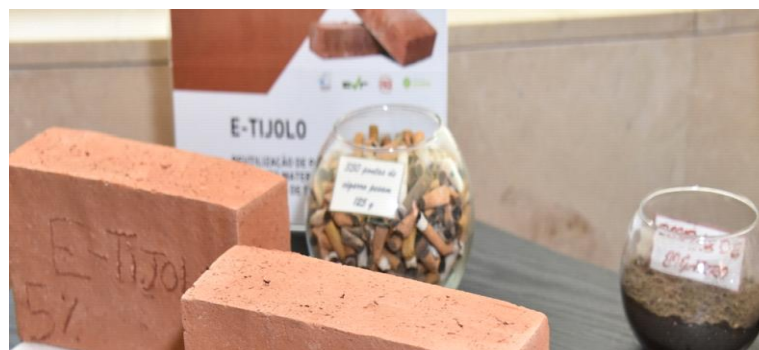
E.TIJOLO – USE OF WASTE IN THE MANUFACTURE OF BRICKS, WITH A REDUCTION IN THE ENERGY
